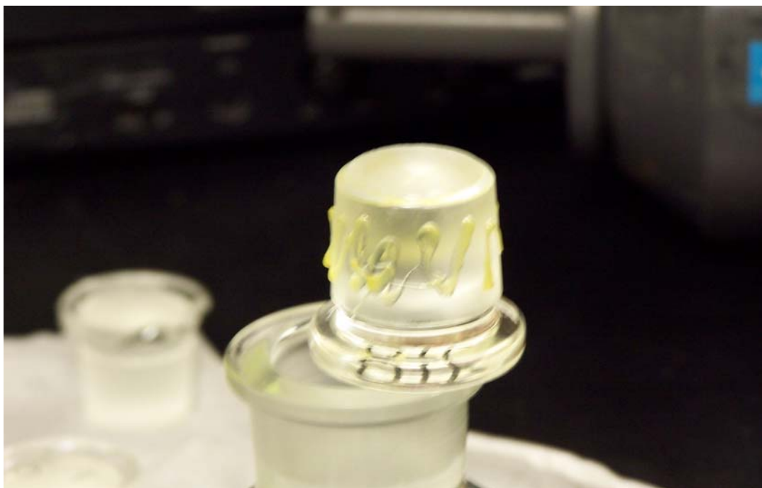
A properly greased glass stopper before insertion into bottle.
