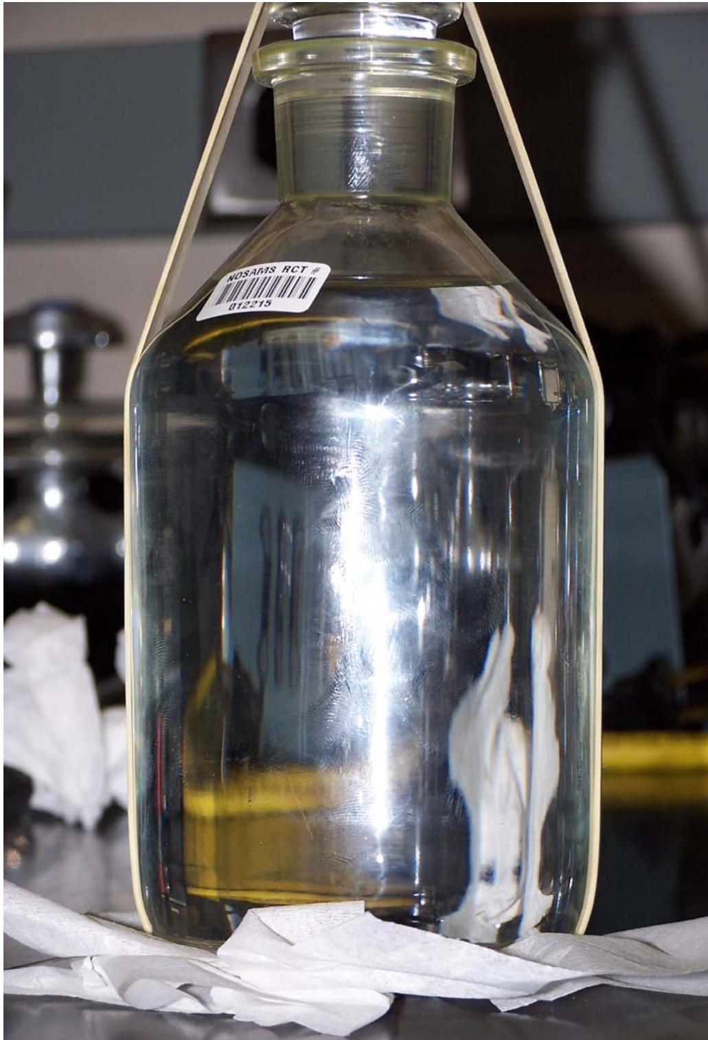
A properly filled and sealed water bottle.
