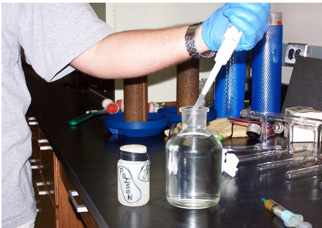
Poison being added to sample. Make sure neck of bottle is dry BEFORE greased glass stopper is inserted.
