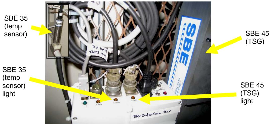
Figure 3. TSG Data Interface Box
